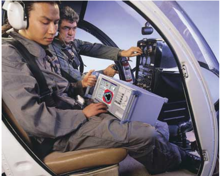
Compact size and independence from local AC supplies make the R&S PSP7 suitable for universal applications. It can be powered from diverse onboard networks – in vehicles, on ships or in aircraft.
